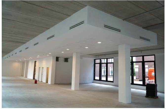
Lowering the structural ceiling height in selected sections for easier (collision-free) installation of suspended ceiling installations – Campus Loddenheide office building, Germany
