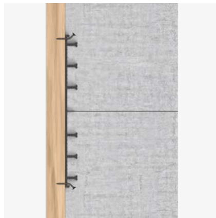
Wall/wall construction joint: Fixed to the formwork.
