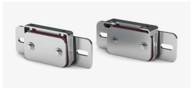
Modification of the JAI types to create dowel variant If it is not possible to secure the JAI elements to anchor channels, custom-designed dowel variants of the elevator insulation JAI can be used. The JAI element is pre-fitted on a dowel plate and then fixed in the shaft with dowels.
