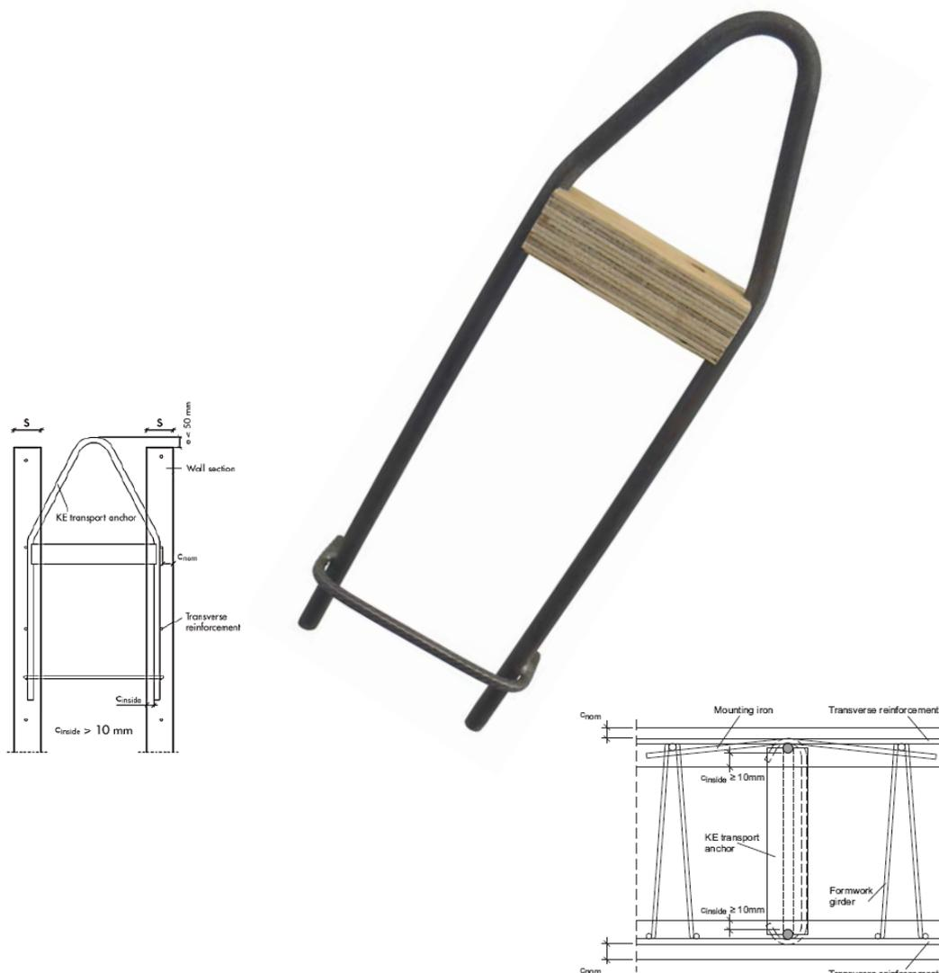
No further description of the KE double-wall transport anchor will be given, attention being drawn to the information in the following figure 2 since it is shown in sufficient detail there.
